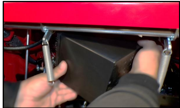
Figure 11 Reinserting Battery into Battery Tray
