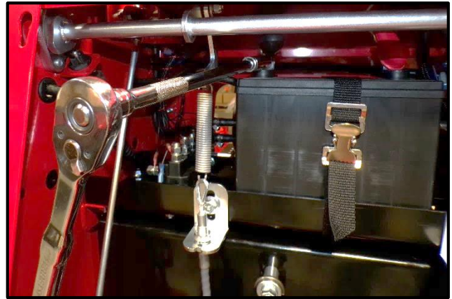
Figure 9 Removing Negative Terminal from Battery
