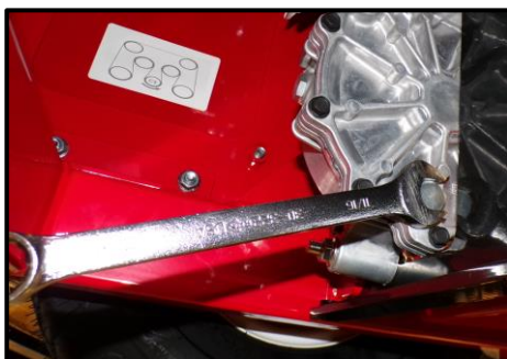
Figure 6 Drain Bolt on Transaxle
