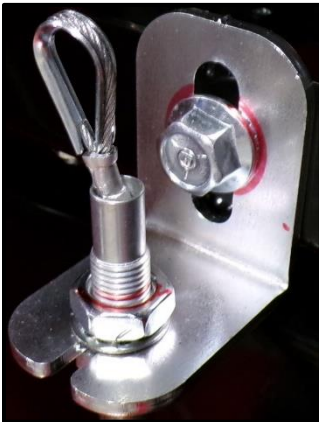
Figure 13 Parking Brake Cable Bracket Location Marked
