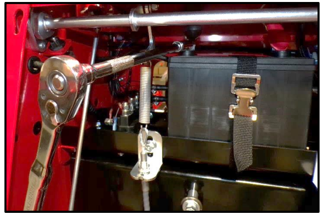
Figure 9 Removing Negative Terminal from Battery
