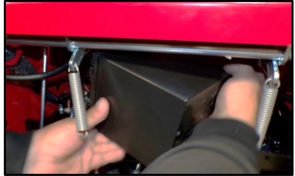
Figure 11 Reinserting Battery into Battery Tray
