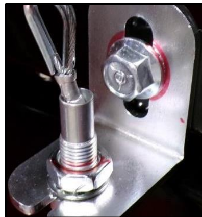
Figure 27 Parking Brake Cable Bracket Location Marked
