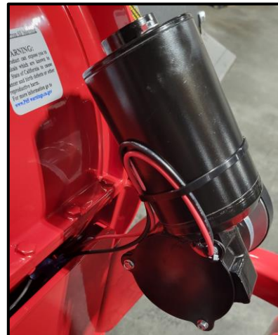
Figure 13 Wires Secured to Rotation Motor
