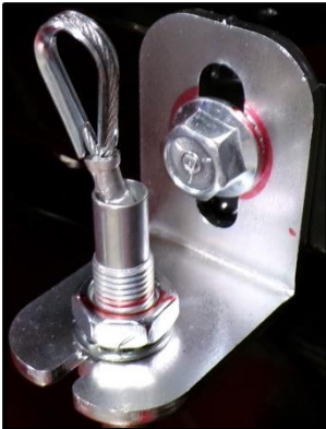
Figure 13 Parking Brake Cable Bracket Location Marked
