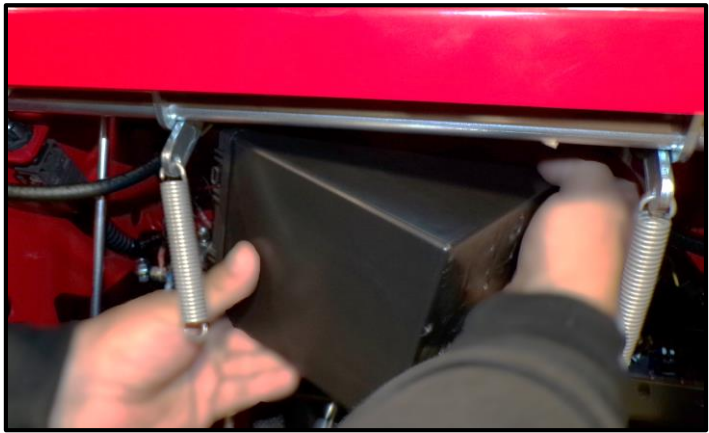
Figure 13 Reinserting Battery into the Battery Tray
