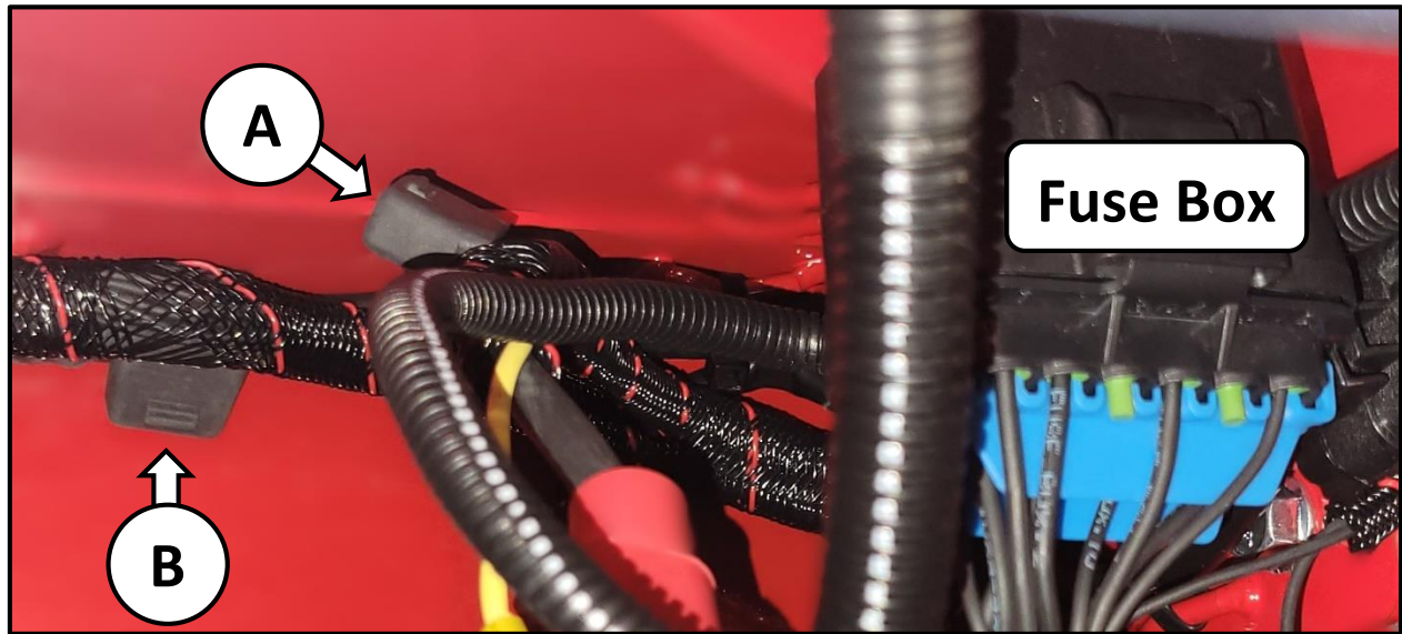
Main Harness Fuse (30A): [A] Fuel Reserve Fuse (10A): [B]
