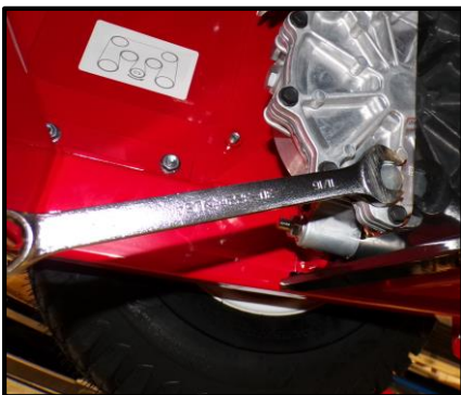
Figure 5 Drain Bolt #1 Location
