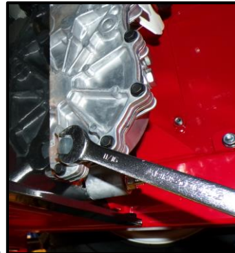
Figure 4 Drain Bolt #2 Location
