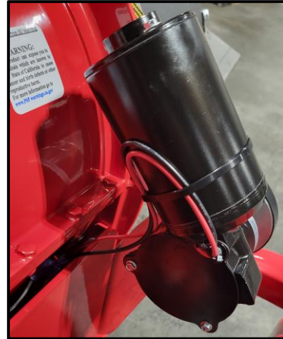
Figure 13 Wires Secured to Rotation Motor
