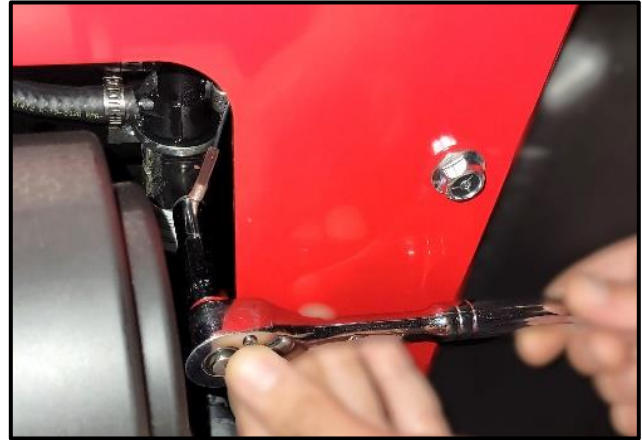
Figure 15 Removing Positive Wire from Fuel Transfer Switch
