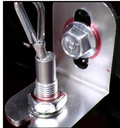
Figure 27 Parking Brake Cable Bracket Location Marked
