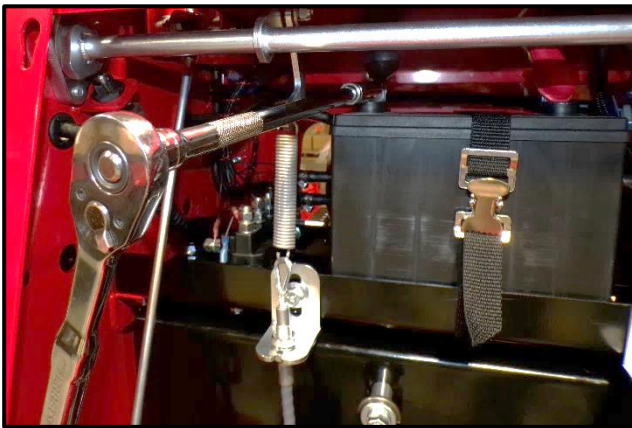
Figure 1 Removing Negative Terminal from Battery
